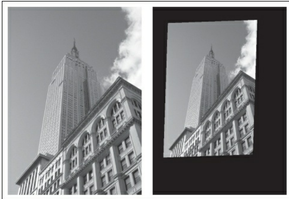
Figure 3-1. An example of warping an image using an affine transform: original (left), image after warping with ndimage.affine_transform() (right).
