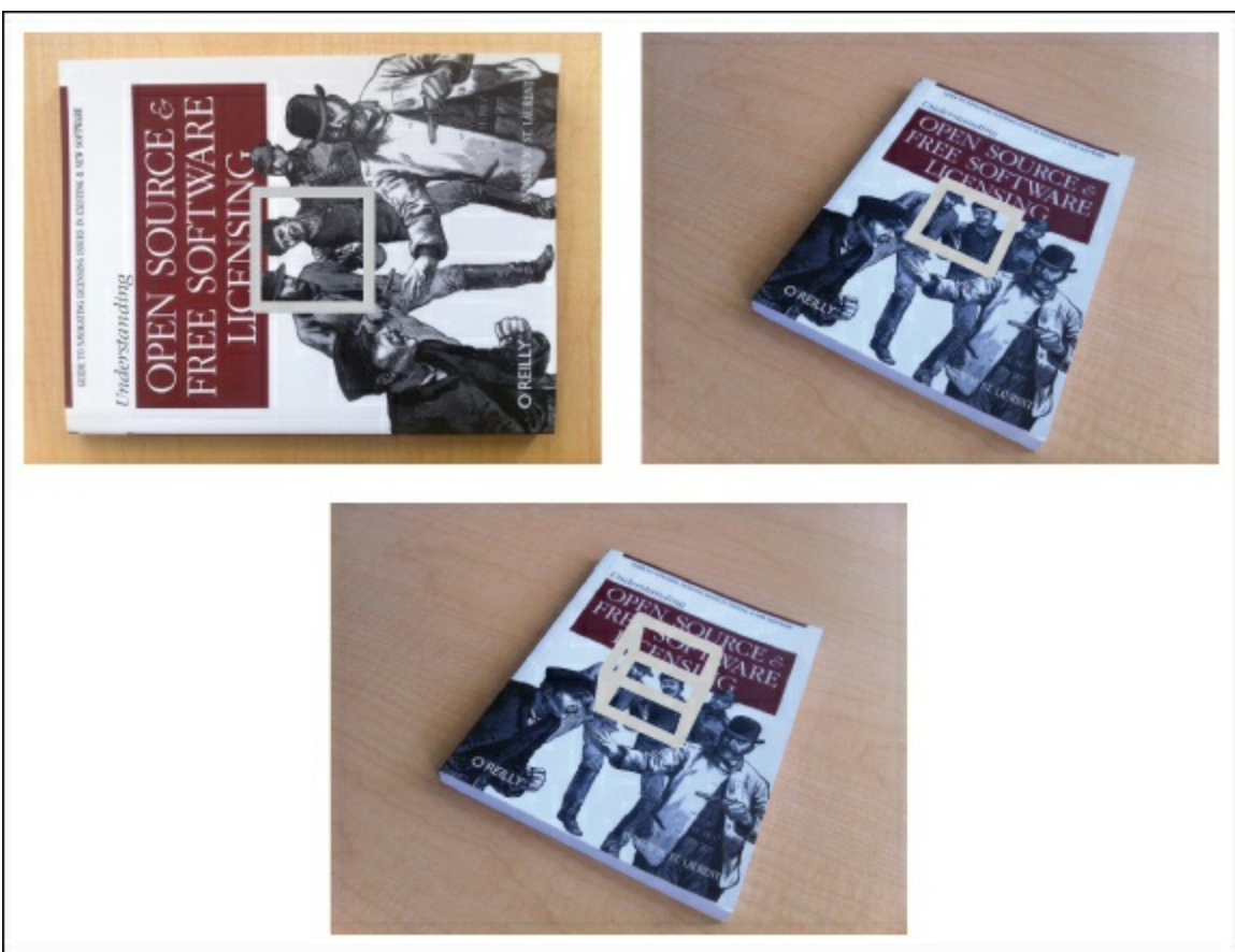
Figure 4-4. Example of computing the projection matrix for a new view using a planar object as marker. Matching image features to an aligned marker gives a homography that can be used to compute the pose of the camera. Template image with a gray square (top left); an image taken from an unknown viewpoint with the same square transformed with the estimated homography (top right); a cube transformed using the estimated camera matrix (bottom).
