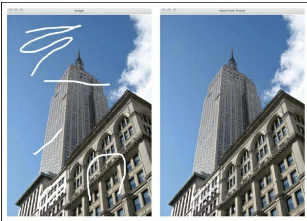
Figure 10-8. An example of inpainting with OpenCV. The left image shows areas marked by a user as “corrupt.” The right image shows the result after inpainting.
