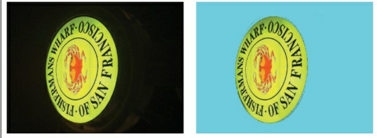
Figure 10-2. Flood fill of a color image. The highlighted area in the right panel marks all pixels filled using a single seed in the upper-left corner.
