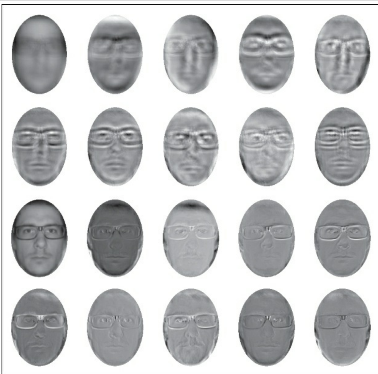
Figure 3-8. Comparing PCA-modes of unregistered and registered images: the mean image and the first nine principal components without registering the images beforehand (top); the same with the registered images (bottom).
