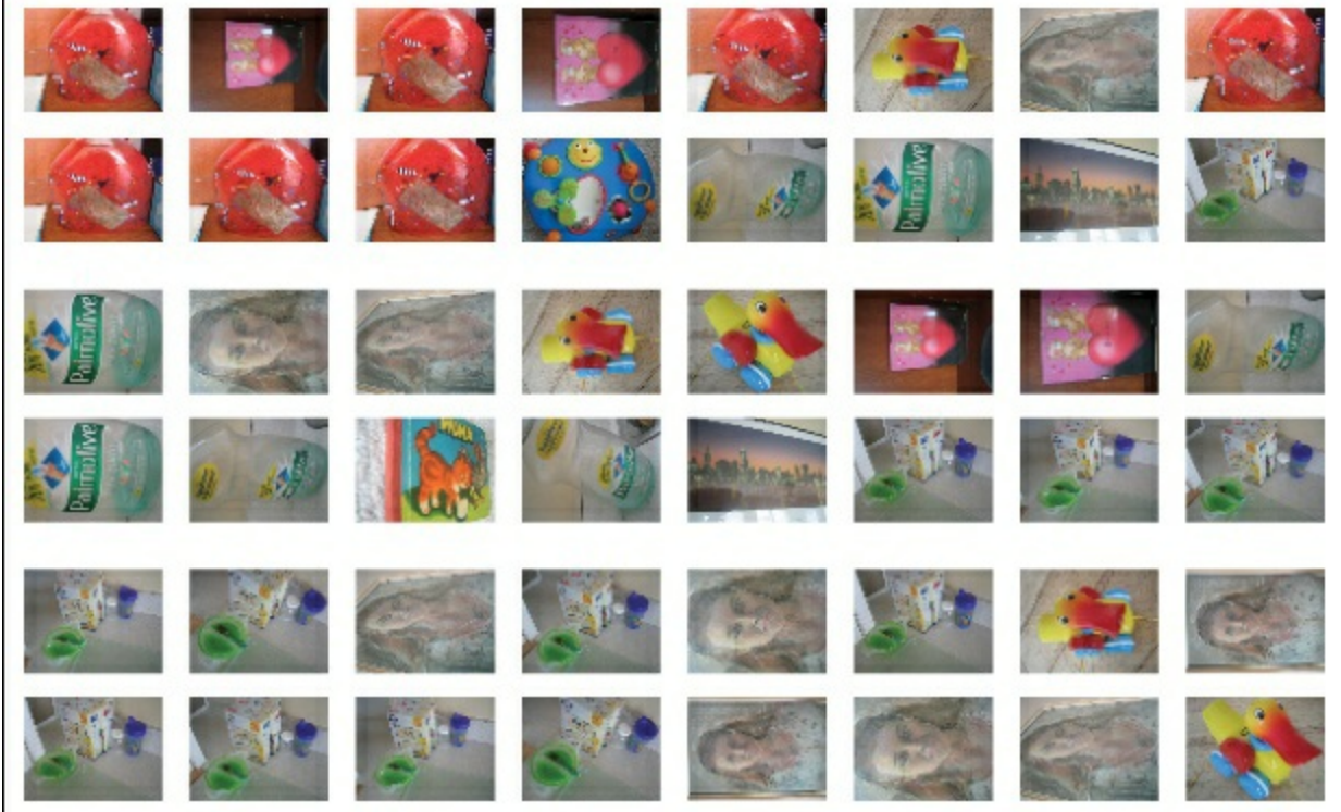
Figure 7-3. Some example search results with re-ranking based on geometric consistency using homographies. For each example, the top row is the regular result and the bottom row the re-ranked result.
