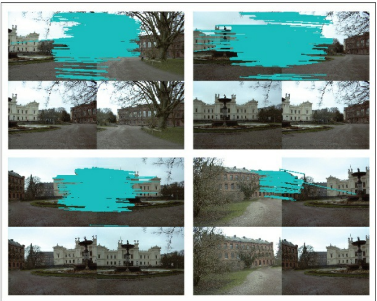
Figure 3-11. Matching correspondences found between consecutive image pairs using SIFT features.
