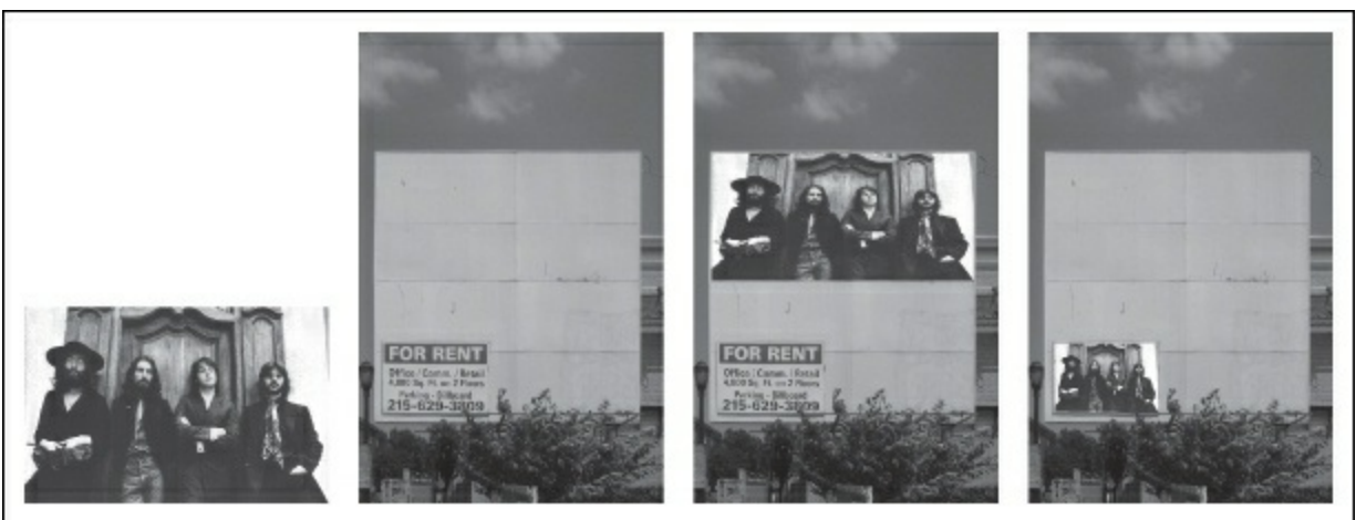
Figure 3-2. An example of placing an image inside another image using an affine transformation.
