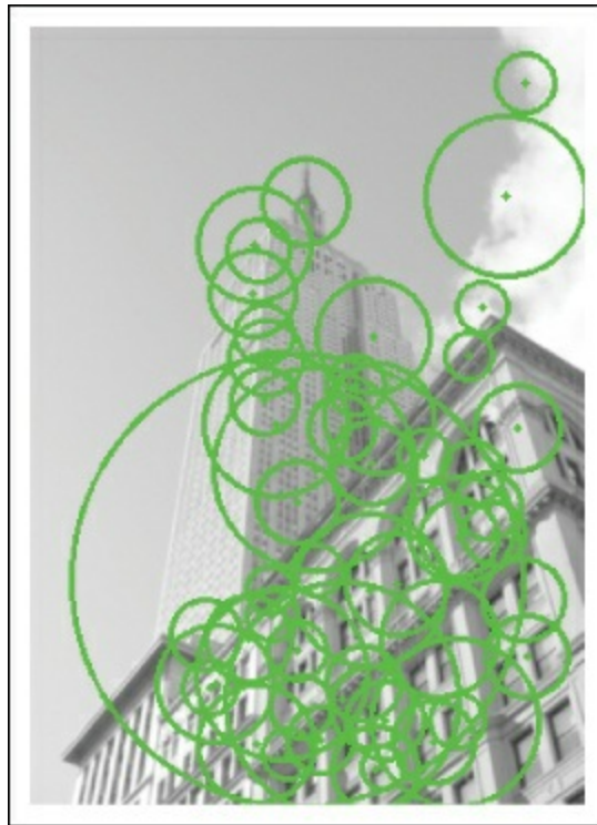
Figure 10-3. Sample SURF features extracted and plotted using OpenCV.
