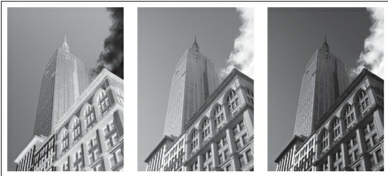
Figure 1-5. Graylevel transforms. Applying the functions in Figure 1-4 : Inverting the image with f(x) = 255 - x (left), clamping the image with f(x) = (100/255)x + 100 (middle), quadratic transformation with f(x) = 255(x/255)^2 (right).
