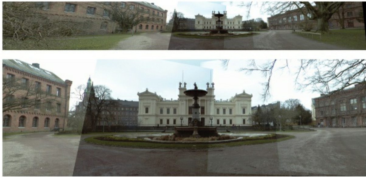
Figure 3-12. Horizontal panorama automatically created from SIFT correspondences: the full panorama (top); a crop of the central part (bottom).
