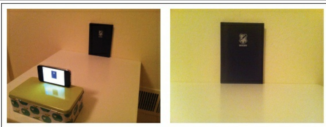
Figure 4-3. A simple camera calibration setup: an image of the setup used (left); the image used for the calibration (right). Measuring the width and height of the calibration object in the image and the physical dimensions of the setup is enough to determine the focal length.
